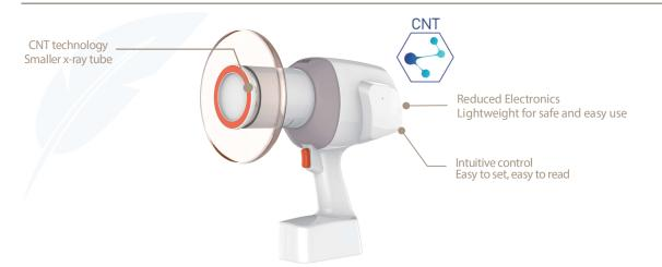
EzRay Air Vet uses carbon nanotube technology instead of conventional x-ray tubes to produce high resolution, diagnostic images. CNT x-ray tubes function more efficiently than traditional tubes by eliminating high temperatures associated with thermionic electron emission required for an x-ray exposure. This technology allows for a compact design as well as image uniformity.
